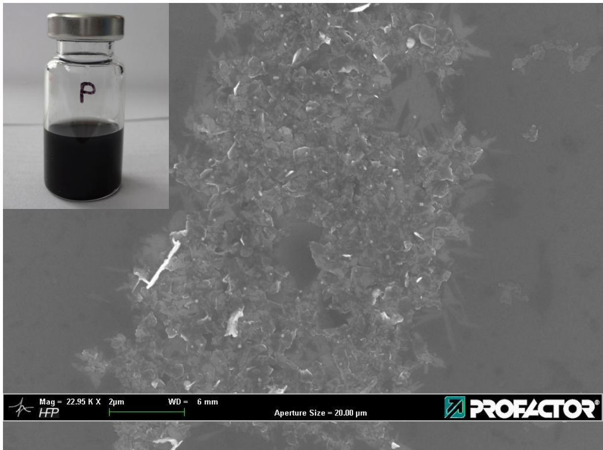
Figure 1 SEM image of graphene/graphite flakes on Si/SiO 2 substrate. Inset: 10 ml-Vial with dispersed flakes in 1-pentanol.
